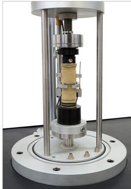
Soil sample fitted with On sample transducers for local strain measurement
