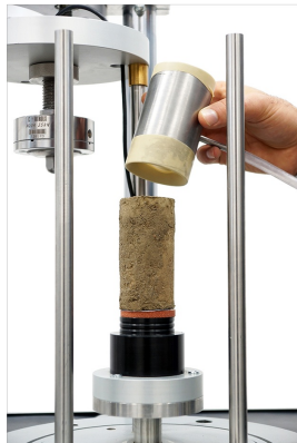
Detail of internal load frame with sample and pivoting crosshead
